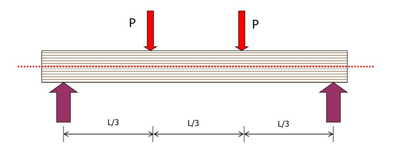
Measure applied load, deflection, beam cross section, and span.
