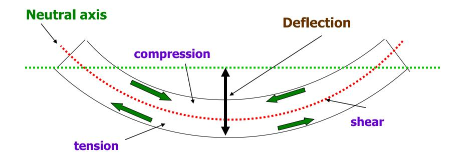
MOE is then calculated using beam dimensions, span, Load, and deflection:
